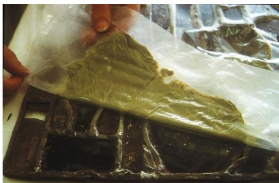
Fig. 3. Removal of the dressing by lifting the Japan paper. Photo: Josep Gri.
